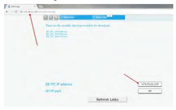
2 HTTP port: Indicates the port for HTTP data transferring. The default is 80 and generally it does not need to be changed. If connecting remotely, it is possible that a firewall will block traffic on this port, in that case contact the IT department for the authorized port. Optionally can be changed to 8080.
