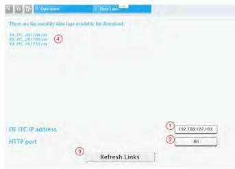
This screen allows the user to retrieve the DE ITC data logs. The data logs are csv files that are created at the end of the month, the name of the file reflects its date, for example: DE\_ITC\_201710.csv is the data log corresponding to October 2017.
